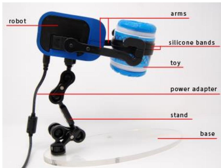
Figure 1. RUBJOY SCHEMATIC [not visible: plastic spacers]
